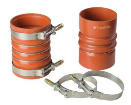
Flexfab's 4000 series CAC hose and clamp kits feature 4-ply silicone coated meta-aramid fabric with stainless steel pressure retention rings. They perform well in extreme temperatures and have all stainless steel spring-loaded T-bolt clamps. The clamps resist salt water and can be used in marine applications.
